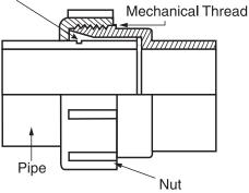
The 3" and 4" joint design differ from smaller versions in that the sealing ridges are located on the fitting and the elastolive extends to the end of the pipe.
