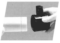
3. Examine the grooving tool to ensure that the cutting blade is fully retracted. Insert the pipe into the grooving tool.
