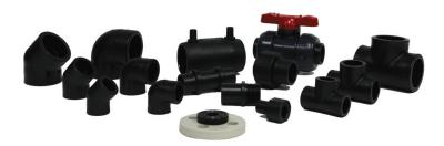
A complete system that includes pipe, fittings, valves, leak detection, injection quills and chemical feed skids, Chem Proline® has a design life expectancy of up to 50 years. Asahi/America's thermally fused Chem Proline® uses no glues and features minimal threaded connections. Asahi/America's Chem Proline® is UV resistant and can be installed above or below ground using socket, butt or electrofusion joining methods.
