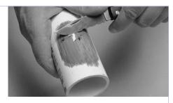
penetration has been made if you can scratch or scrape a few thousandths of an inch of the primed surfaces away.
