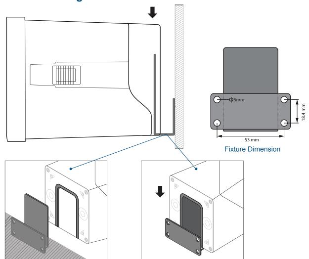
Install bracket on the wall first
